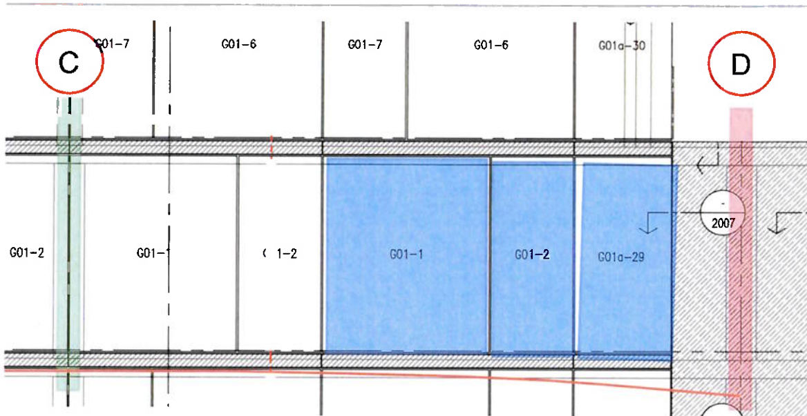
Figure 12 EWS-001 glass rotating due to differential settlement of one column (South elevation)
