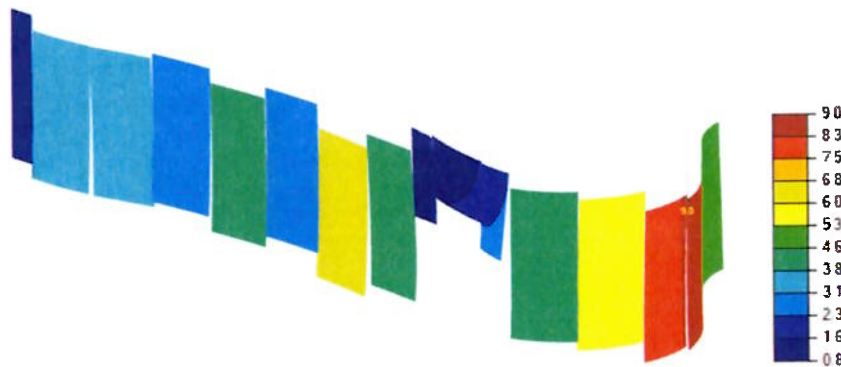
Figure 24 EWS-006 Total displacement of glazing panels including movement due to self-weight
